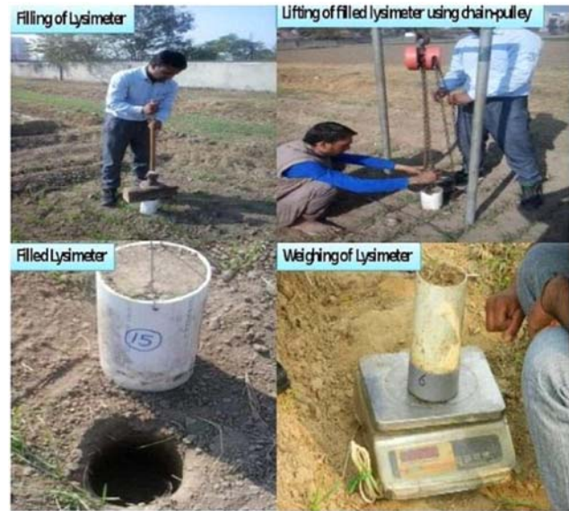
Figure 1. Technique of measuring soil evaporation viz. mini-lysimeters for measuring soil evaporation in the field a. Fitting of lysimeter; b. Removal of filled lysimeter using chain-pulley arrangement; c. Filled lysimeter; d. Weighing of filled lysimeter on daily basis to have day to day evaporation in differently established plots (Bhatt, 2015)
