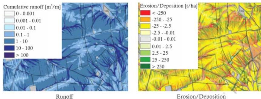
**Figure 3.** Runoff and soil erosion output maps of EROSION 3D model (*Source:* Schmidt and Werner, 2020)
