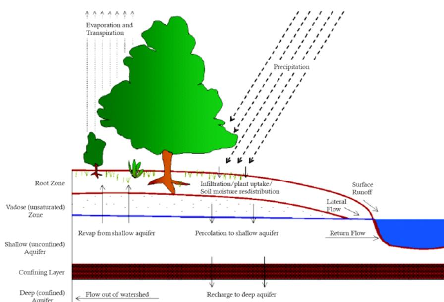
Figure 2. Representation of hydrologic cycle in SWAT model (Source: Neitsch *et al.*, 2011)
