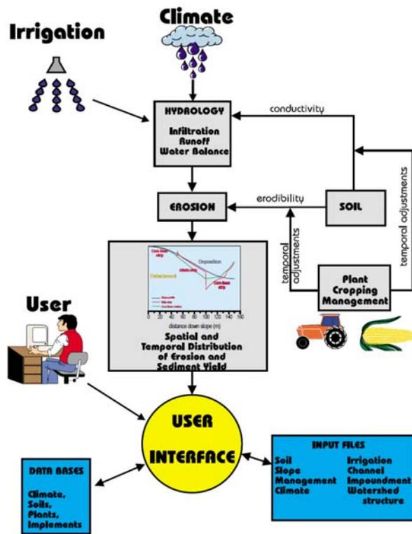
Figure 1. Flow chart for WEPP runoff and erosion prediction model (Source: Flanagan *et al.*, 1995)
