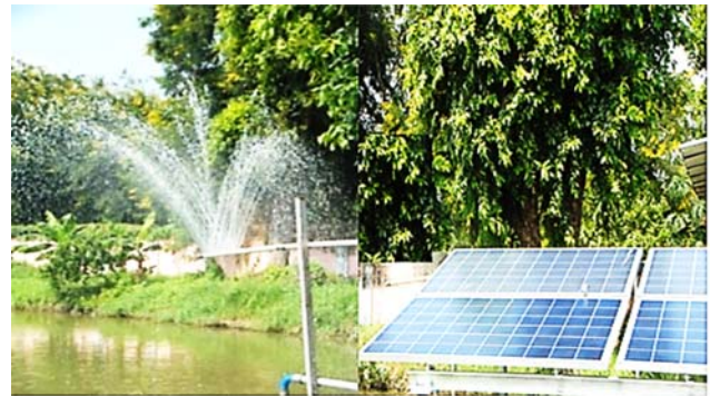
Figure 4. The schematic diagram and operational view of solar aerator at ICAR-RCER, Patna
