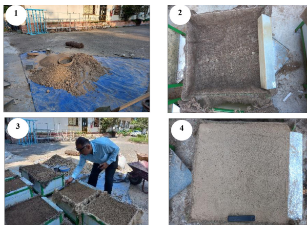
Fig. 1. Steps in preparing experimental plots Sieving soil (1), pouring pumice and placing a layer of hemp sack in the plots (2), preparation (3), and a sample of the prepared plot (4)
