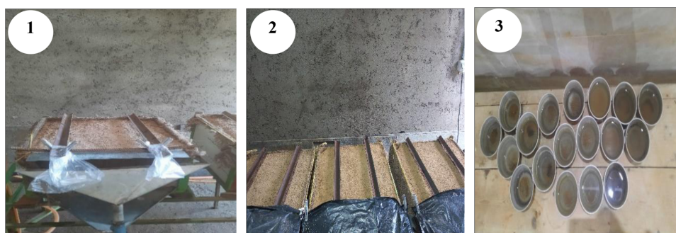
Fig. 2. Steps in measuring splash erosion Installation of splash gutters (1 and 2), sediment washed from gutters (3)
