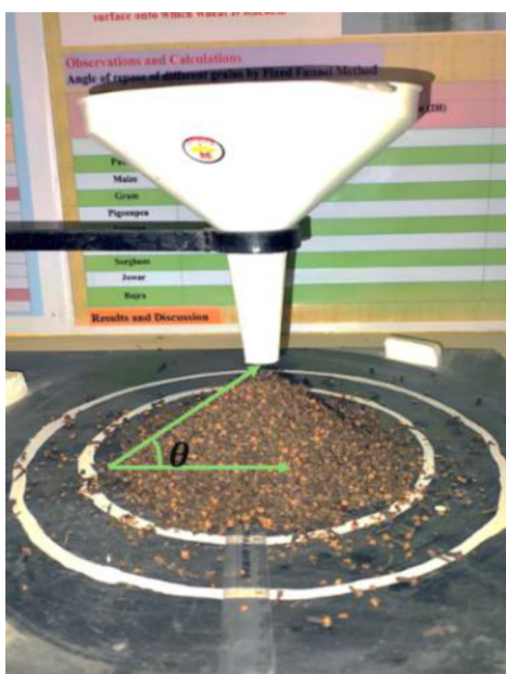
Fig. 3. Measurement of the angle of repose of clove buds
