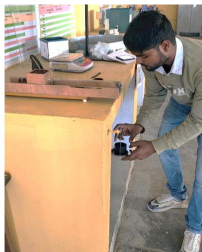
Fig. 4. Measurement of the angle of external friction of clove buds
