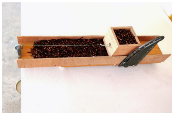
Fig. 5. Measurement of the angle of internal friction of clove buds
