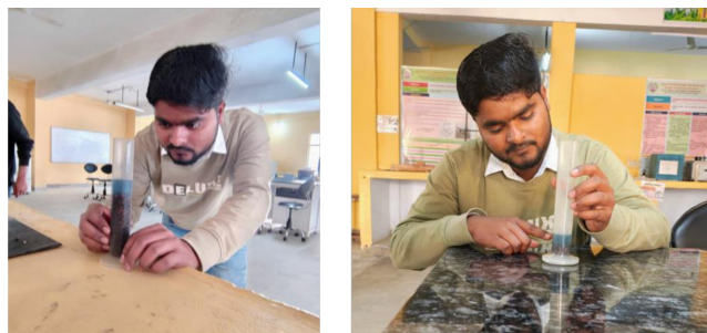
Fig. 2. Liquid displacement technique to determine true density of clove buds Porosity
